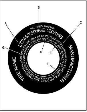
(A) Tire Size: The tire size code is a combination of letters and numbers used to define a particular tire's width, height, aspect ratio, construction type and service description. See the "Tire Size" illustration later in this section for more detail.
